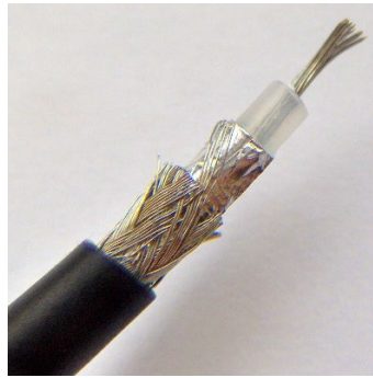
Power substation at the Pueblo of Acoma, New Mexico, close up of the coaxial cable (the most common transmission line) and operational transmission lines on the Gila River Reservation
