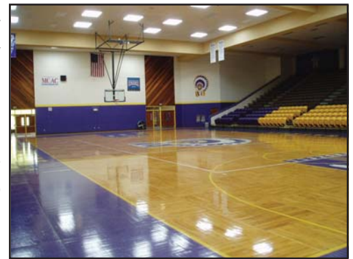
Skylights provide sufficient illumination for Haskell's gymnasium without using electric lighting.
